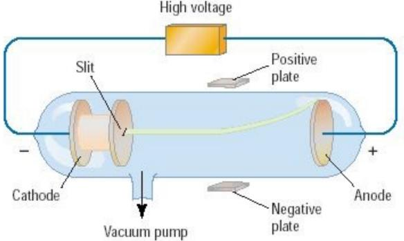
Cathode ray tubes pass electricity through a gas that is contained at a very low pressure.
